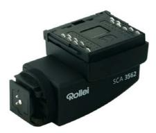
To shoot with a portable flash in TTL mode, you need a Rollei 3562 Adapter (Leaf part # 604-00212) and an SCA 3002 system flash. A Rollei 356 Adapter (Leaf part # 604-00211) is also available for shooting with the SCA 300 flash system for film. Presently, only Metz makes flashes that can be used in TTL mode on the Leaf AFi camera system.
